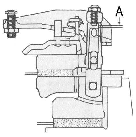
Flywheel measurement from clutch mounting surface to disc friction surface: 1.750'' Verify PTO Gap (A) using the smooth shank of a 1/16'' drill bit as a gauge.
