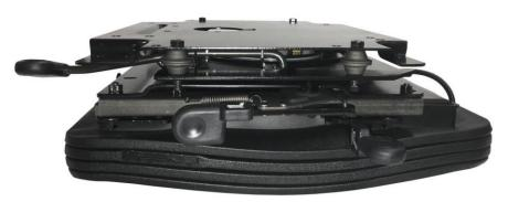
6. Bolt seat to seat plate using (2) washers as spacers between seat and seat plate and  $5/16" \times 1/2"$  bolt per hole
