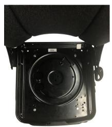
7. Use screws to reattach the seat bottom
